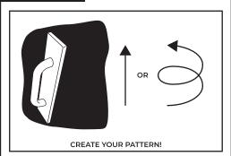
A short while after applying DaVinci Gamazine Decorative Plaster to the desired surface run the plastic floating trowel over the Plaster in a vertical or circular motion in order to achieve the desired effect.
