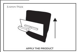
Once you've loaded your Stainless Steel Plastering Trowel, Apply the product onto the desired surface swiping from bottom to top. Aim to keep the application as thin as 3-4mm for the best coverage results.
